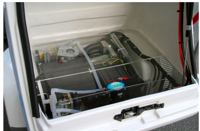
Fig. 11. Fuel cell/battery hybrid power system installed on the cargo of the light vehicle.
