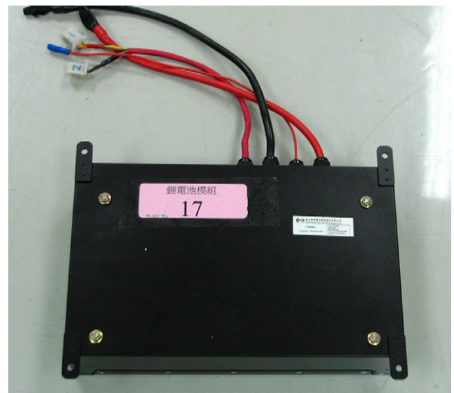
Fig. 8. Photo of lithium-ion battery package.
